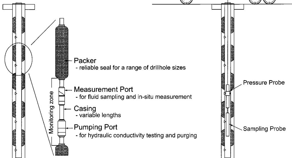
Fig. 3. Multi-packer system (Westbay, Ltd., Canada) showing sampling procedure.
